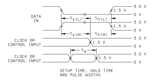
FIGURE 3. Test circuit and switching waveforms.
