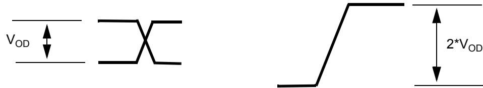
Figure 19 - Differential Voltage Parameter
