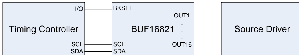
Figure 20. Gamma Control Block Diagram
