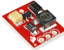
The NCP1402 is a 3.3V DC-DC converter. The breakout board will accept voltage inputs between 1 and 3 Volts (such as 1 or 2 AA batteries) and output a constant, low ripple 3.3V output capable of sourcing up to 200 mA. This board is great for supplying power to 3.3V sensors or providing 3.3V from a single AA battery.
