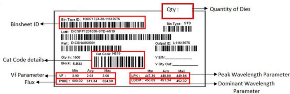
Fig 13. Example of a bin sheet label for LUXEON FlipChip Royal Blue.
