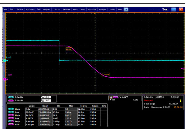
Figure 10-3. Recessive to Dominant Propagation
