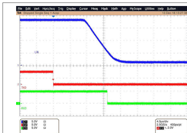
Figure 10-11. Recessive to Dominant Propagation Delay
