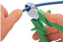
Cutting a cable.
