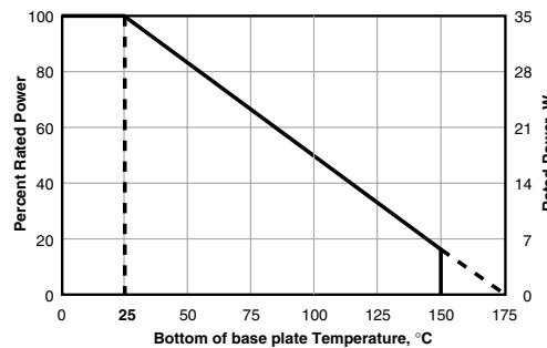
**Derating (thermal resistance):**  $0.23\text{W}/^\circ\text{C}$  ( $4.28^\circ\text{C}/\text{W}$ ). The case temperature is to be used for purposes of establishing the applied power limit. The case temperature measurement must be made with a thermocouple contacting the center of the component mounted on the designed heat sink. Thermal grease should be applied properly.
