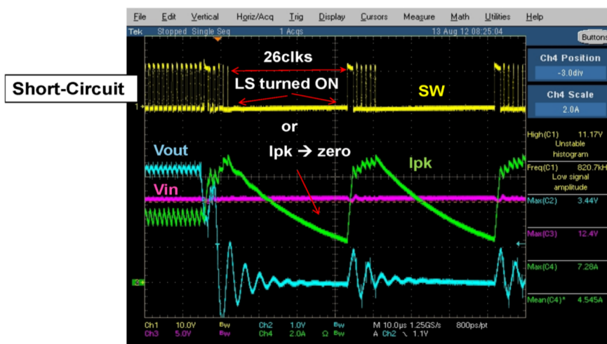
Figure 18. Constant current protection triggering hiccup mode
