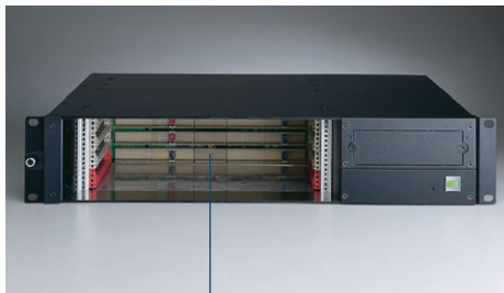
4-slot backplane with H.110 CT Bus
