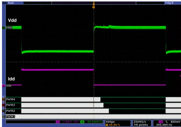
Figure 40: Wide View of Phase Shed/Add
