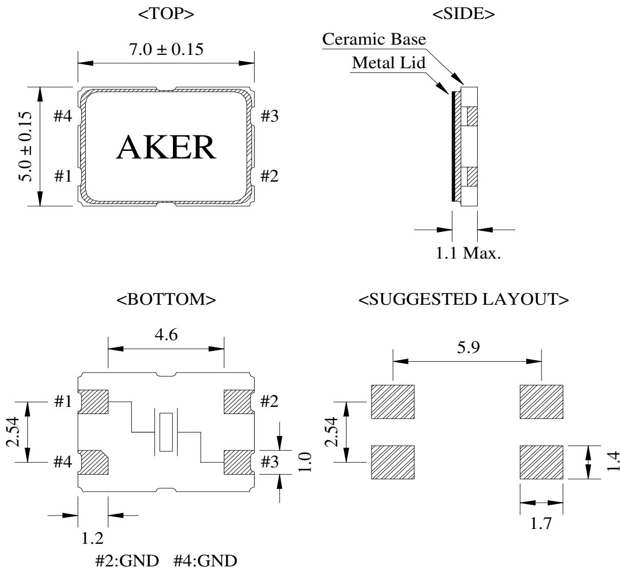
Package is Seam Sealed Ceramic-Metal.
