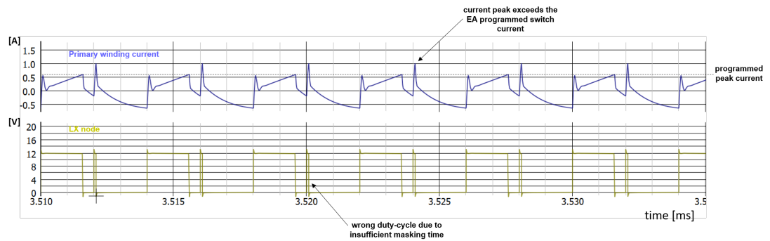
Figure 13. Simulation with appropriate masking time (330 ns)
