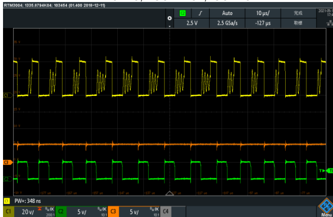
Operating at 65W Flyback Application VIN= 115VAC, VOUT= 15V, IOUT= 3A
