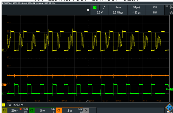
Operating at 65W Flyback Application VIN= 115VAC, VOUT= 20V, IOUT= 3.25A
