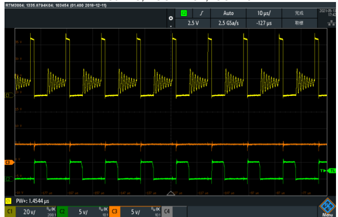
Operating at 65W Flyback Application VIN= 230VAC, VOUT= 15V, IOUT= 3A
