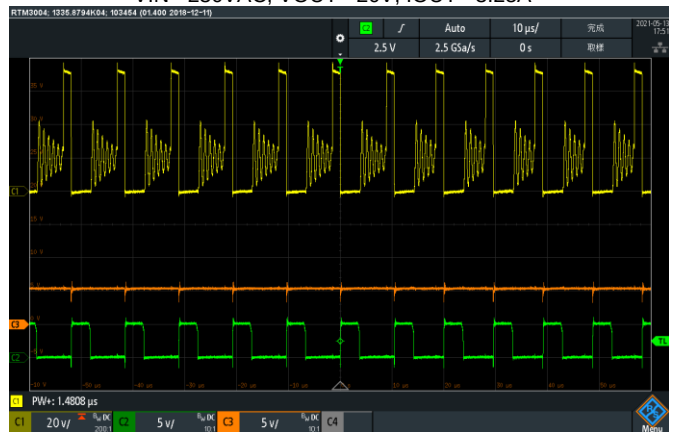
Operating at 65W Flyback Application VIN= 230VAC, VOUT= 20V, IOUT= 3.25A
