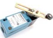
Series HDLS Plug-in: Low Temperature Version; Side Rotary; 2NC 2NO DPDT Snap Action; 0.5 in - 14NPT conduit
