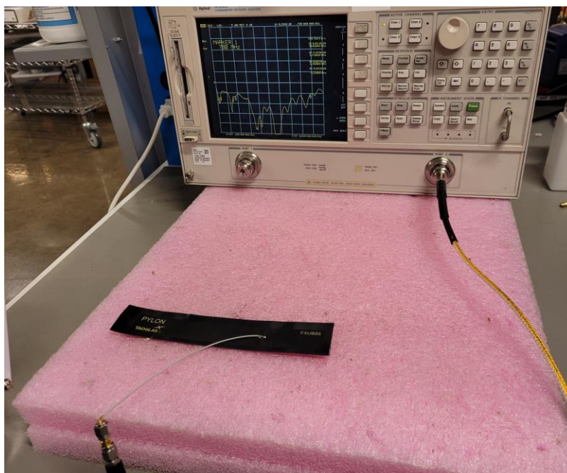
Return loss Test Setup of the FXUB85.54.0150C
