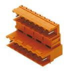
Dimensionally stable, angled, codable 2-tier male connector from the Unimate range of plugs with integral aid to prevent wrong connections. Available with open or closed sides. Fixing blocks can be attached to the closed version. The solder pin length of 3.2 mm has been optimised for wave soldering. Supplied in cardboard box.
