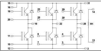
It is recommended to connect a decoupling capacitor between pins 31 & 2 to reduce switching overvoltages, if DC Power is connected between pins 15, 16 & 12. Pins 15 & 16 must be shorted together.
