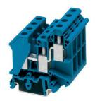
Feed-through terminal block, nom. voltage: 800 V, nominal current: 57 A, connection method: Screw connection, 1 level, Rated cross section: 10 mm², cross section: 0.5 mm² - 16 mm², mounting type: NS 35/7,5, NS 35/15, NS 32, color: blue
