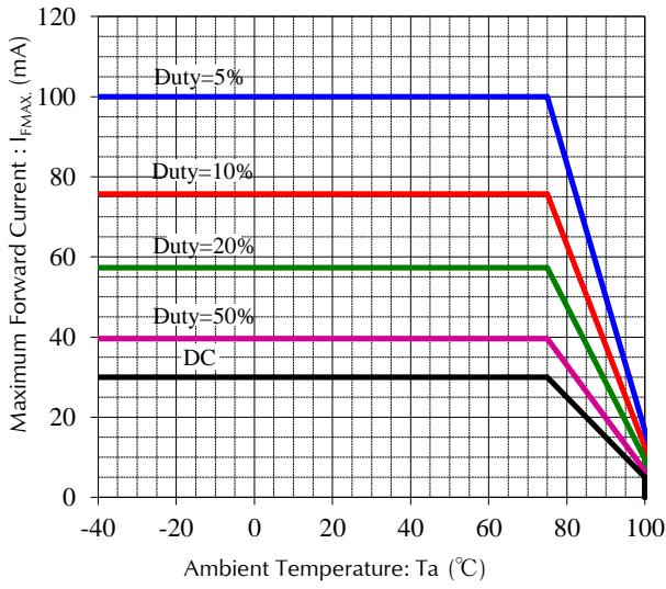
Duty Cycle vs. Max. Forward Current
