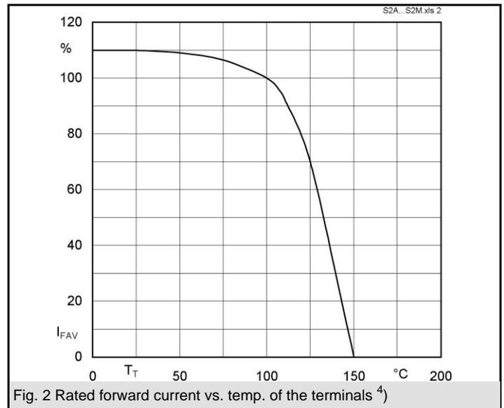
Fig. 2 Rated forward current vs. temp. of the terminals <sup>4)</sup>
