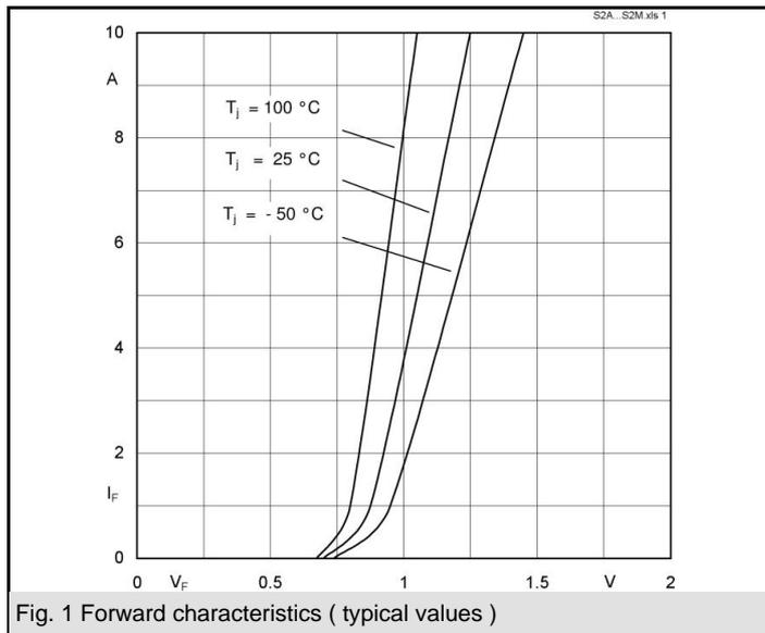
Fig. 1 Forward characteristics ( typical values )
