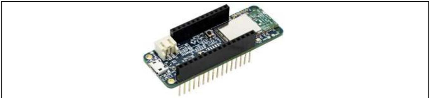
**Figure 2** CYSBSYSKIT-DEV-01 rapid IoT connect developer kit
