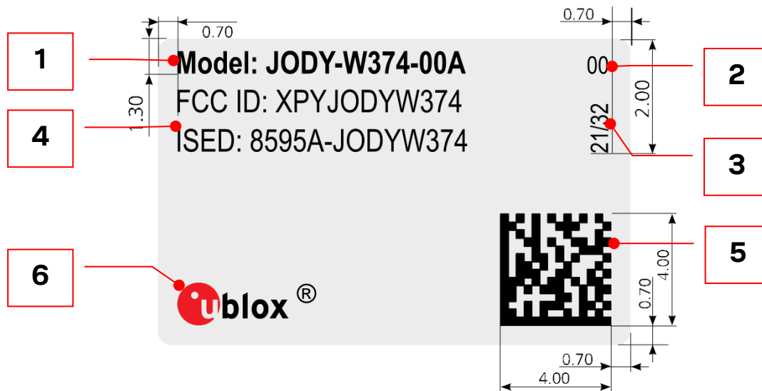
Figure 20: JODY-W3 series sample label
