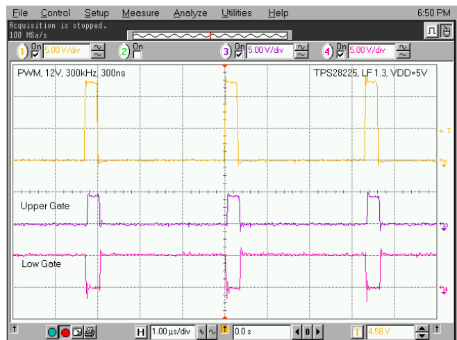
Figure 23. 12-V PWM Pulse at V_{DD} = 5 V
