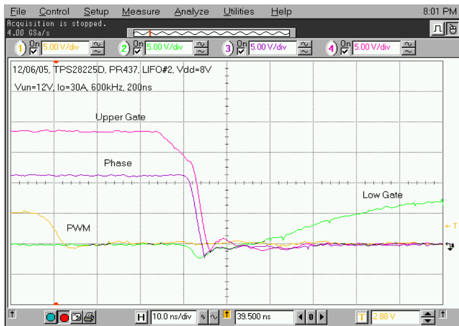
Figure 30. Phase Falling Edge Switching Waveforms (10ns/div) of the Power State in Figure 27
