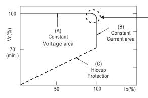
In the constant current region, the highest voltage at the output of the driver depends on the configuration of the end systems.
