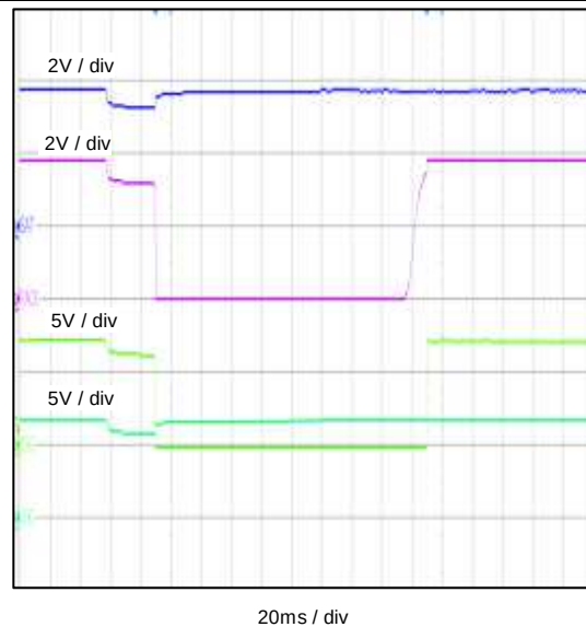
Figure 16. Overcurrent in Discharge Protection Set and Clear
