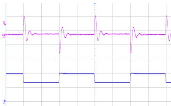
Figure 5 Dynamic response for 25% load step (50% ~ 75% ~ 50%) and 1A/μs slew rate, (2ms/div), see Figure 10 for test configuration; CH2-output voltage (200mV/div); CH1-output current (10A/div)
