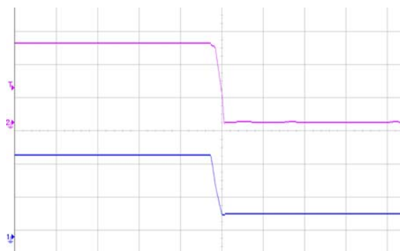
Figure 7 Output voltage shut down by power off, (50ms/div), see Figure 10 for test configuration; CH2-output voltage (5V/div); CH1-input voltage (20V/div)
