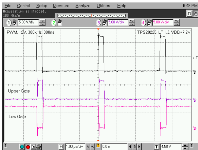
Figure 22. 12-V PWM Pulse at V_{DD} = 7.2 V
