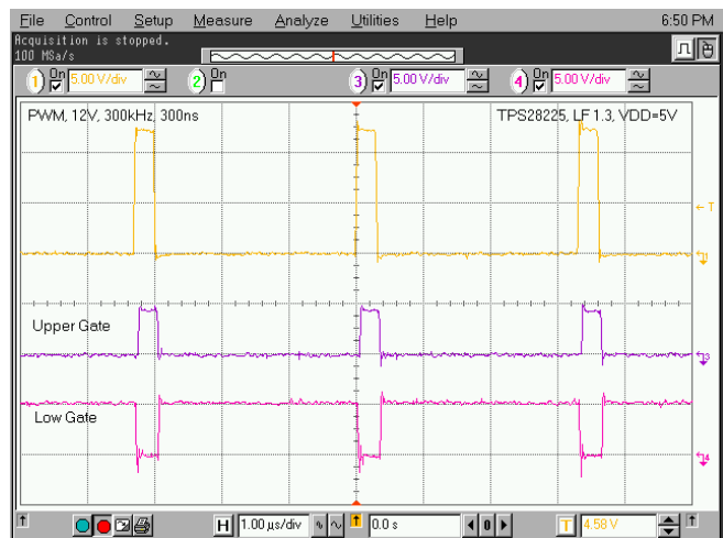
Figure 23. 12-V PWM Pulse at V_{DD} = 5 V
