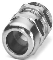
Cable gland, material for screw connection: Brass, nickel-plated, application: Standard, external cable diameter 11 mm ... 17 mm, shielding: no, connecting thread: M25 x 1.5, color: silver, with O-ring
