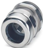
Cable gland, material for screw connection: Brass, nickel-plated, application: EMC, external cable diameter 11 mm ... 16 mm, shielding: yes, connecting thread: M25 x 1.5, color: silver, with O-ring
