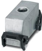
Sleeve housing B24, with double locking latch, material: Die-cast aluminum, salt water resistant, cable outlets: 1, straight, 1x M25, height: 60 mm, cable gland: none, Standard
