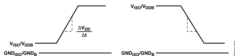
Figure 21. Transient Immunity Waveforms, Output Supplies
