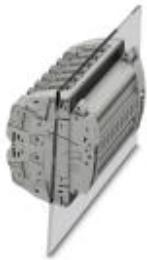
Test terminal strip, Connection method: Ring cable lug, Number of connections: 24, Number of positions: 12, Width: 130.4 mm, Height: 70.1 mm, Color: gray, Mounting type: Wall mounting
