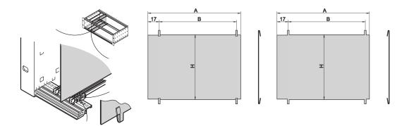
The divider plate enables the user to create a separate area inside a subrack or case. The plate can be clipped into the perforation of the horizontal rails. The subracks or cases have to be disassembled if the plate will be assembled.
