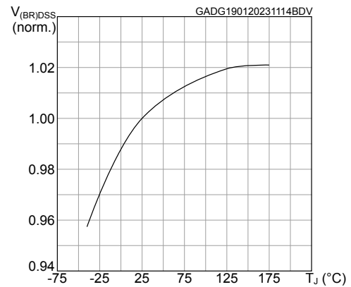
Figure 8. Normalized breakdown voltage vs temperature
