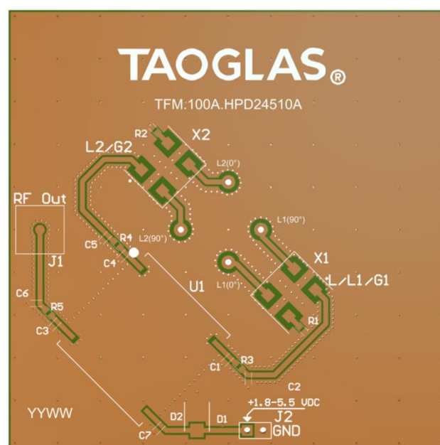
Top Side ( HP24510A placement on 70x70mm PCB)
