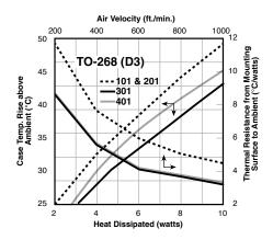
Final thermal performance is highly dependent on the thermal characteristics of the PCB. It is possible to see a 50% drop in temp rise in natural convection with a thermally improved PCB.
