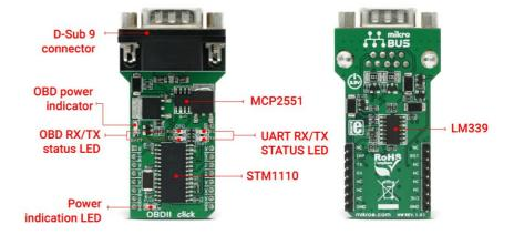
The standard prescribes a set of defined PIDs or Parameter IDs to communicate with the vehicle onboard computer (ECU) and return values from the corresponding locations of the vehicle's controller network, related to a specific PID. There are 10 modes of operation described in the latest
