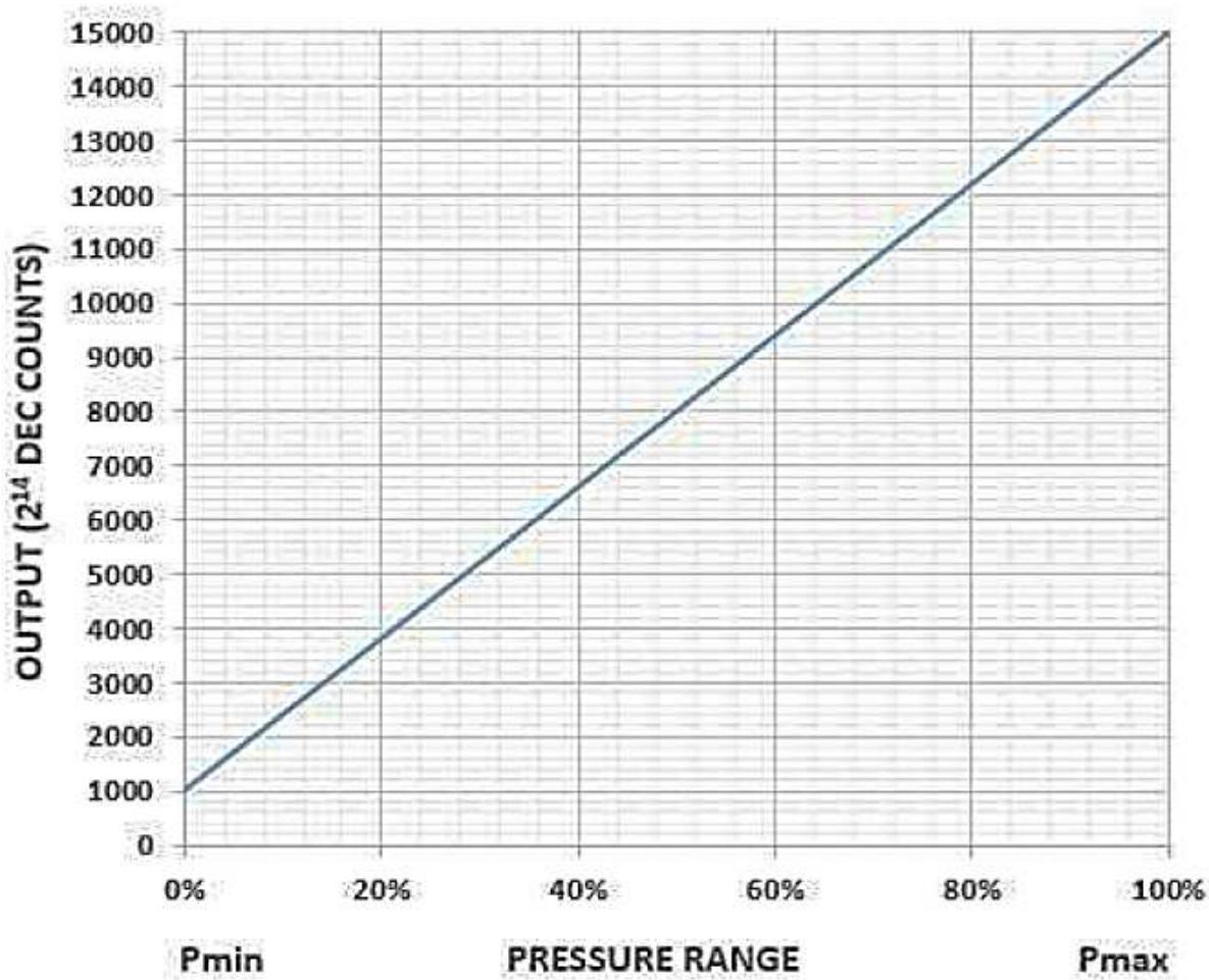
$$\text{OUTPUT (DECIMAL COUNTS)} = \frac{15000-1000}{\text{Pmax} - \text{Pmin}} \times (\text{Papplied} - \text{Pmin}) + 1000$$
