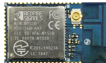
LGA Module (AA1) 27 mm x 16 mm
