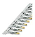
Crimp contact, Socket, rolled, Taped product, number of pieces per reel: 10000, contact diameter: 1 mm, crimp range: 0.22 mm $^2$  ... 0.56 mm $^2$ , Item is lead-free in accordance with RoHS II without Exemption 6c (Pb < 0.1 %)
