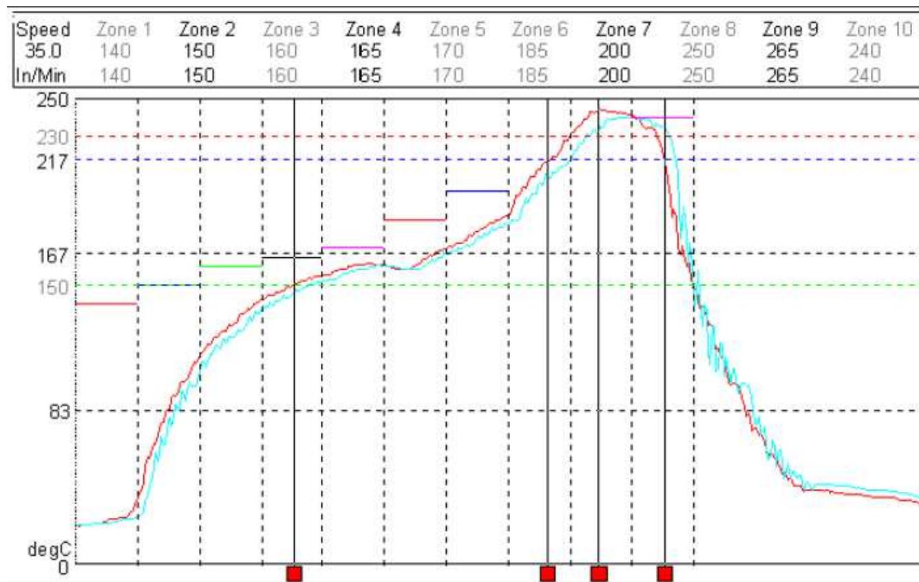
Figure 35. Recommended Solder Reflow Temperature Profile
