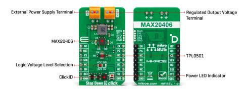
As mentioned, the Step Down 9 Click uses the TPL0501 and its 3-Wire SPI serial interface to communicate with the host MCE, supporting clock frequency of up to 25MHz. The voltage quality can be monitored by observing the PGOOD signal over the PG pin of the mikroBUS™ socket. The enable EN pin is an input for circuit activation, active with a HIGH logic state.
