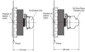
\* These are the dimension from the front of the panel when the Switch Unit is attached.
