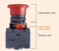
If the sliding operation of the lock lever is insufficient, the operation unit may not function properly when needed, even if pushed. With the lock-lever-linked contact function, if the sliding operation of the lock lever is insufficient, the original NC contact will turn to a NO state when the operation unit is not pushed, making it possible to detect errors from the state of the contact.
