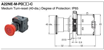
$\textbf{Note:} \ \ \textbf{Unless otherwise specified, a tolerance of $\pm 0.8$mm applies to all dimensions.}$
