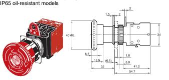
Switch dimensions when mounted to a 2NO (2NC) one-piece switch block
