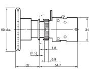
Note: Unless otherwise specified, a tolerance of ±0.8 mm applies to all dimensions.
