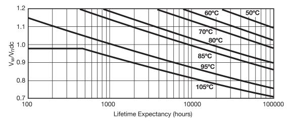
Vw = Permanent working or operating DC voltage.
