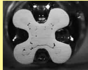
Crimp-cross section HARTING crimp profile
