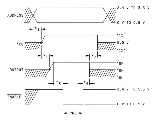
FIGURE 7g. Programming voltage waveforms during programming for circuit G.
