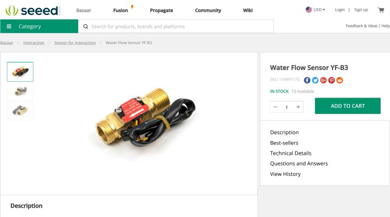
Water flow sensor consists of a copper body, a water rotor, and a hall-effect sensor. When water flows through the rotor, rotor rolls. Its speed changes with different rate of flow. The hall-effect sensor outputs the corresponding pulse signal. This one is suitable to detect flow in water dispenser or coffee machine.
