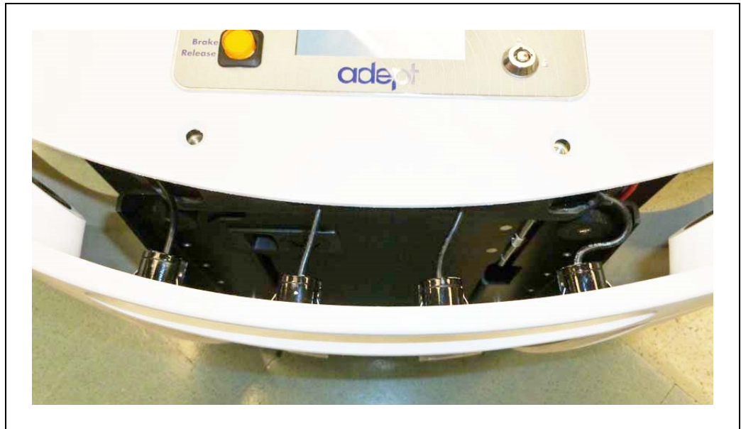
Figure 8-2. Sonar Leads, with Connectors Still in Chassis
