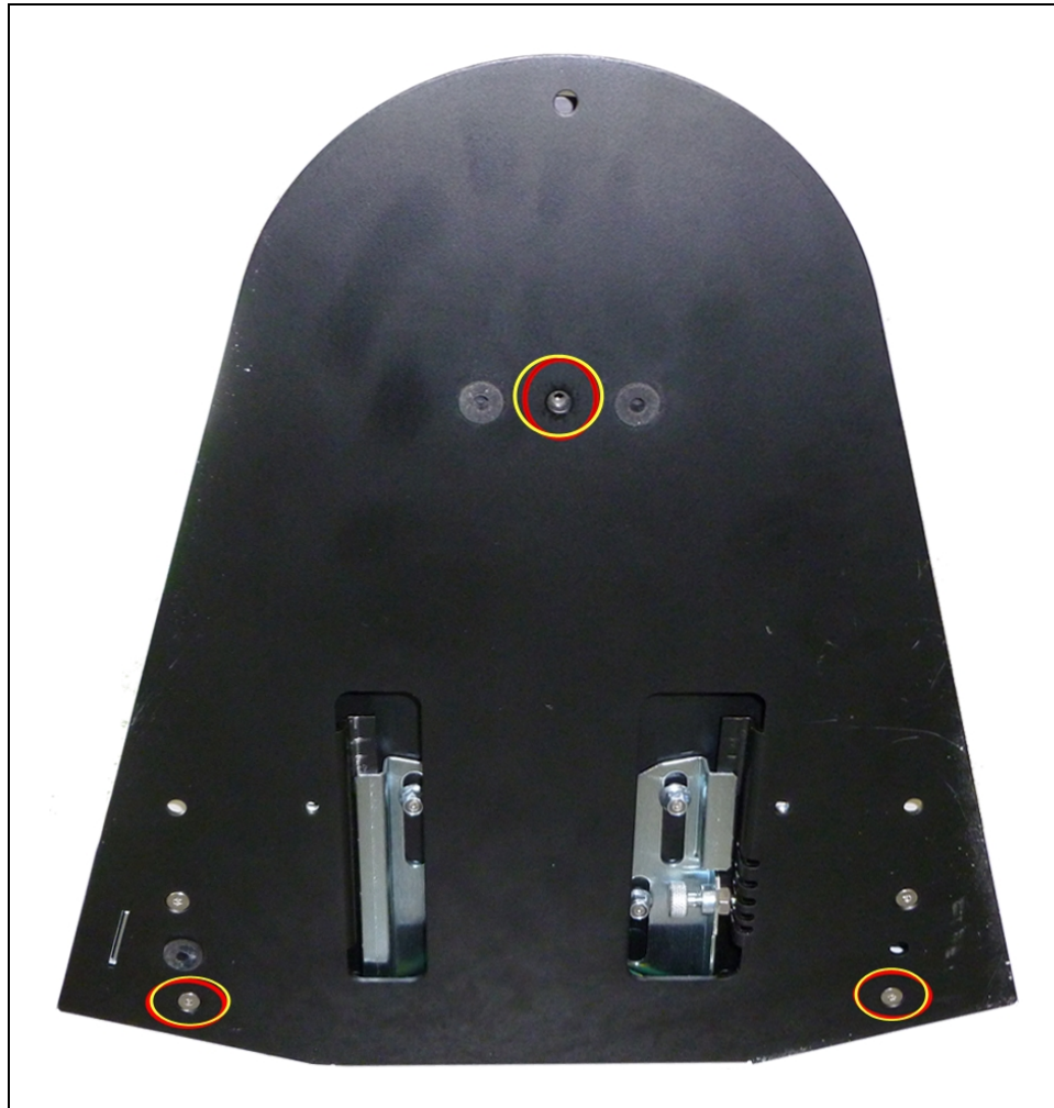
Figure 2-10. Underside of Docking Station Foot, Showing Screw Locations
