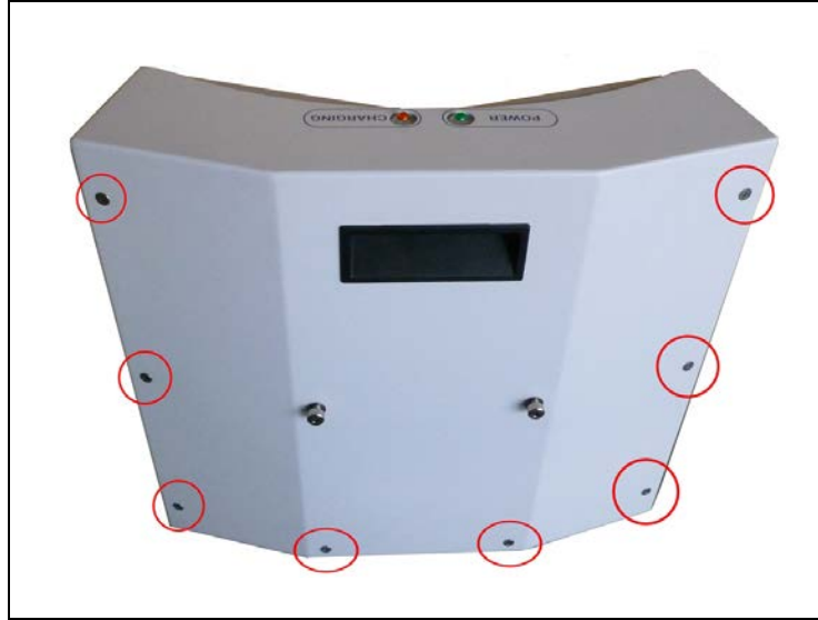
Figure 8-11. Docking Station Rear Cover Screws (8 of 10)
