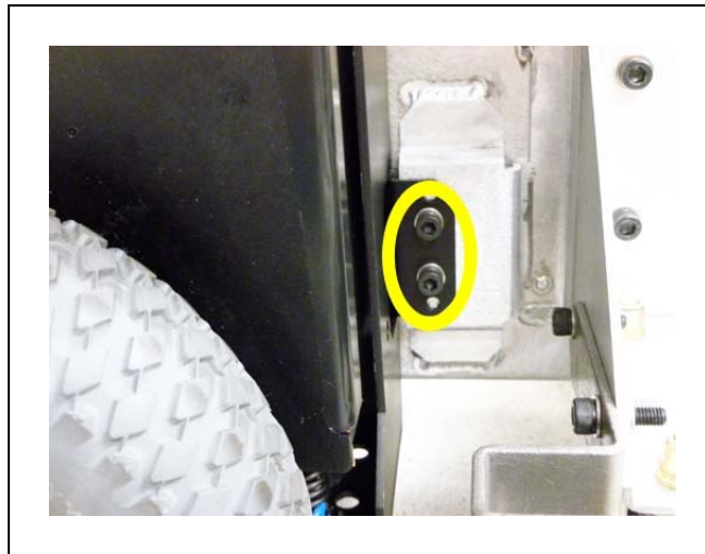
Figure 8-16. Mounting Screws at Bottom-Right of Drive Assembly
