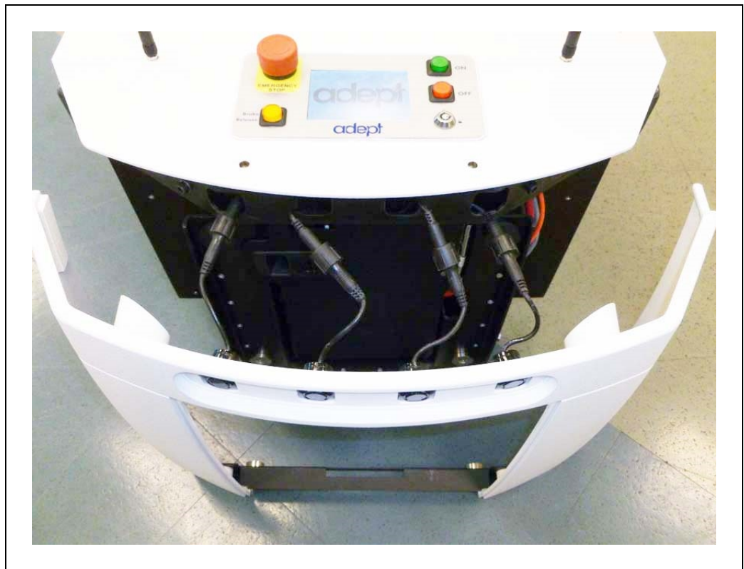
Figure 8-3. Sonar Connectors, with Connectors Exposed
