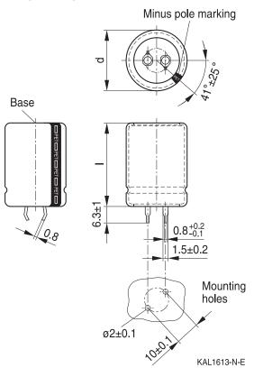
Snap-in terminals, length (6.3 ±1) mm. Also available in a shorter version with a length of (4.5 - 1) mm. PET insulation is marked with "PET" on the sleeve. Safety vent on the case wall.
