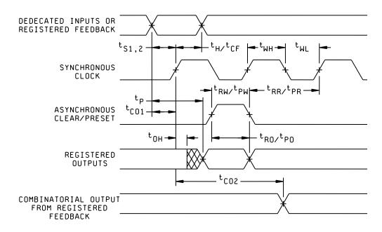
FIGURE 4. Switching waveforms.
